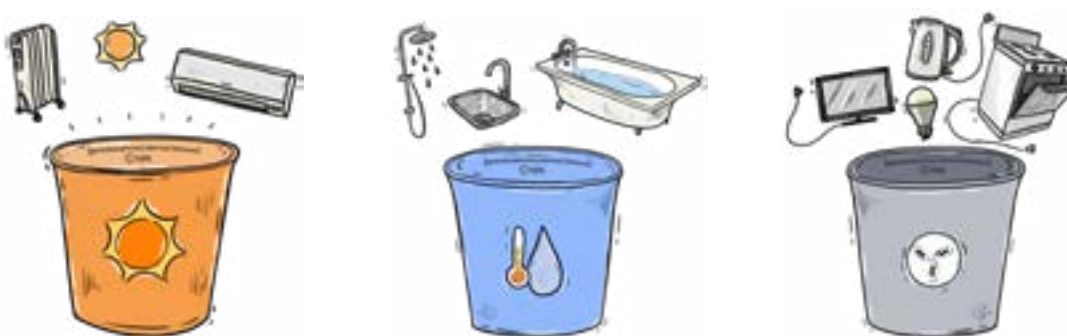
Figure 1. The “3 buckets” concept explains where energy is used in a house. From left to right: the “healthy” bucket (heating, cooling and ventilating); the “hot water”; and the “lights & appliance” buckets (Source: HPA)
